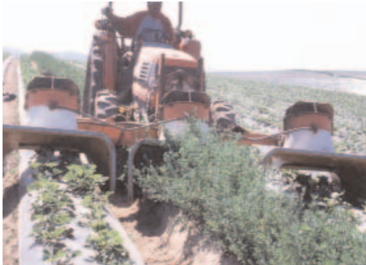
Using the bug vac to collect WTPB from an alfalfa trap crop adjacent to organic strawberries.
