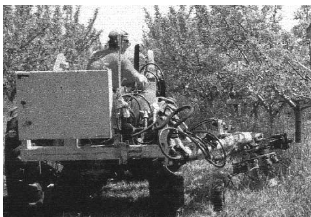
Shallow cultivation with a weed badger at Ricker Hill Orchards in Turner, Maine. Ricker Hill is a 600-acre orchard with a 100-acre organic block. The farm is 200 years old, owned and managed by several generations within the Ricker family.
