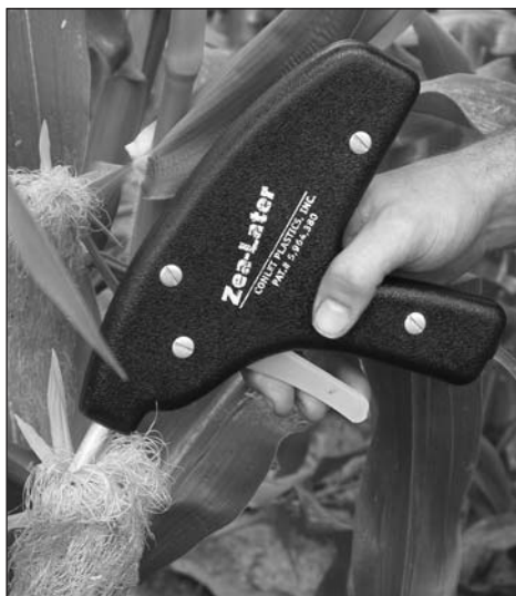
Zea-later™ applicator being used to apply 0.5 ml of oil/Bt to silking corn.
