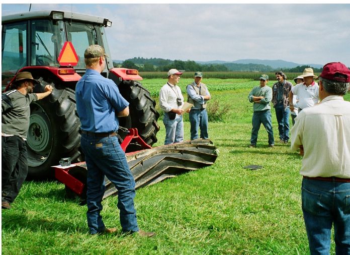
A roller-crimper can be used to terminate cover crops while leaving behind residue that can provide mulch for the following crop. Photo credit: Mark Schonbeck.
