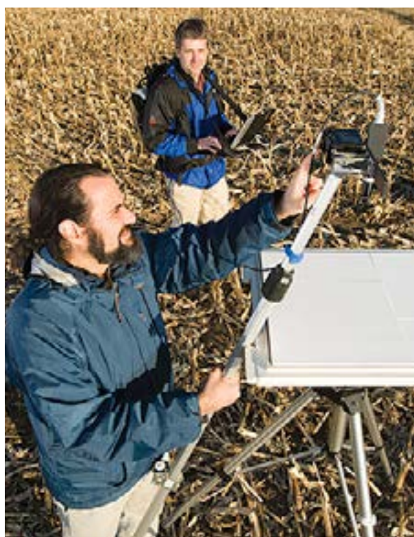
Soil scientist Guy Serbin (left) and remote sensing specialist Any Russ calibrate a portable spectroradiometer over a white panel prior to measuring the reflectance of the crop residues and soils in a cornfield. These ground-based reflectance measurements are used to develop remote sensing tools for assessing soil tillage intensity using satellite and aircraft imagery. Photo by Peggy Greb.
