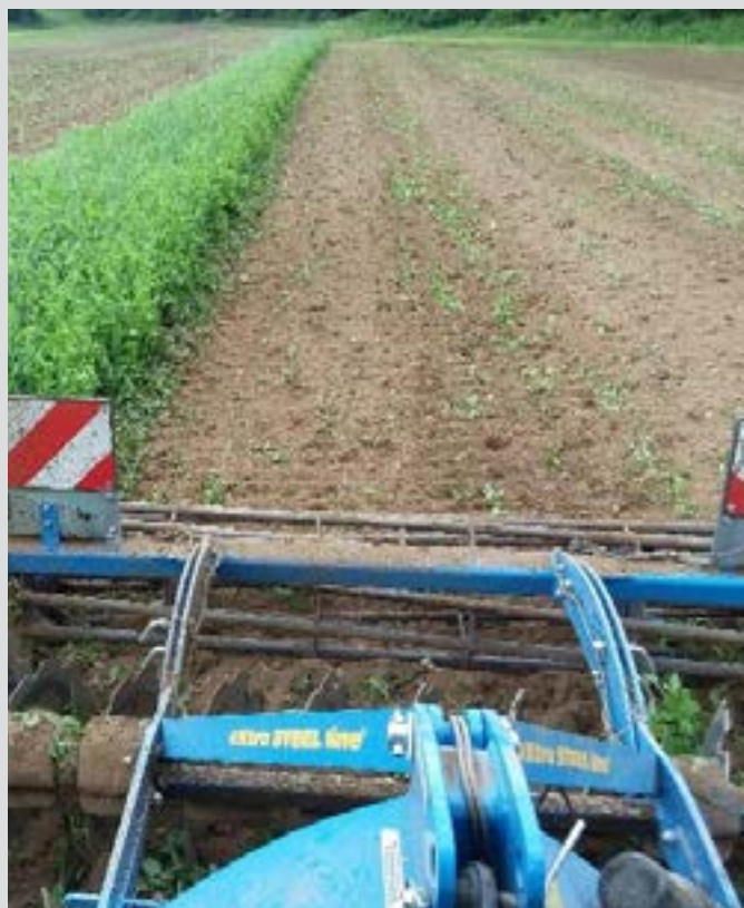
Figure 6. For most tillage operations, Burnt Rock Farm uses a 2.5 meter (8 ft) Farmet Softer high-speed disk equipped with independently sprung, compound-angled, notched disks and a depth-setting rolling basket in the rear. Working 3-4 inches deep at a forward speed of 7-8 mph, the disk chops and incorporates flail-mowed cover crops (left) and makes a satisfactory bed for transplanting in two passes 10 days apart. Winter-killed cover crops require only one pass (right). Because the disk works best in moist soil, Justin incorporates mid-summer covers after a rainfall.
