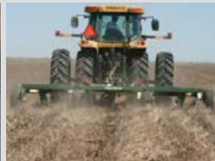
Figure 9. The blade plow or sweep plow undercutter terminates cover crops and weeds by severing root crowns just below the surface, leaving residues in place and most of the soil profile undisturbed. This tool requires just the right soil moisture level, as wet conditions allow the vegetation to regrow, while very dry conditions prevent the tool from penetrating sufficiently to kill the cover crop. "It works about 50% of the time for terminating the green fallow," Doug said. "My fallback option is the speed disk." Photos by Drew Lyon, U. Nebraska.
