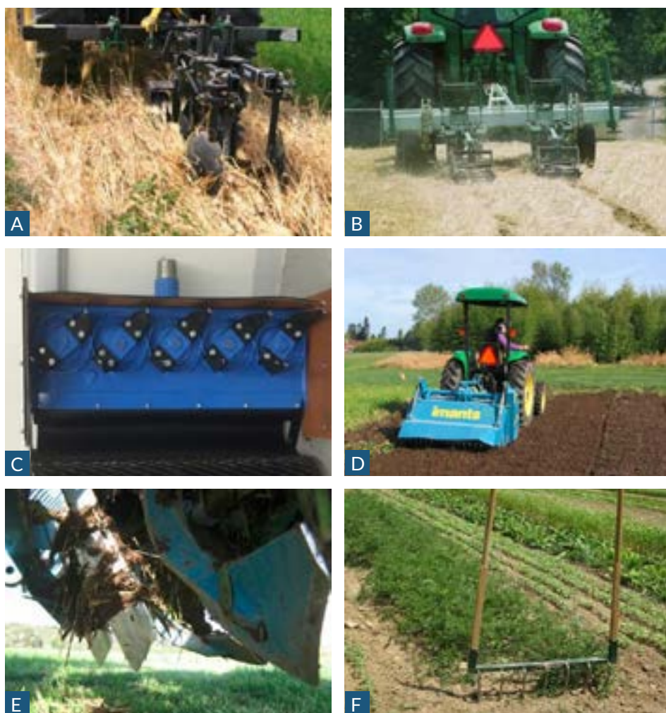
Figure 1. Some tools that organic farmers use to reduce intensity of soil disruption while getting the job done include strip tillers that leave 70-80% of the soil surface undisturbed (A,B), rotary harrow used to work the top 1 – 3 inches (C), reciprocating spader for deep non-compacting tillage (D, E), and broadfork, a manual tool used in small scale operations to loosen bed tops (F).
