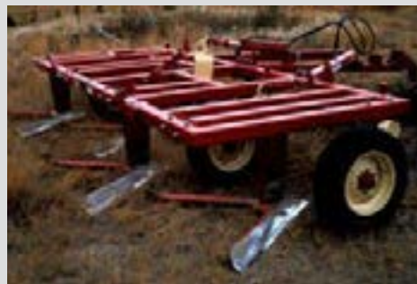
Figure 9. The blade plow or sweep plow undercutter terminates cover crops and weeds by severing root crowns just below the surface, leaving residues in place and most of the soil profile undisturbed. This tool requires just the right soil moisture level, as wet conditions allow the vegetation to regrow, while very dry conditions prevent the tool from penetrating sufficiently to kill the cover crop. "It works about 50% of the time for terminating the green fallow," Doug said. "My fallback option is the speed disk." Photos by Drew Lyon, U. Nebraska.
